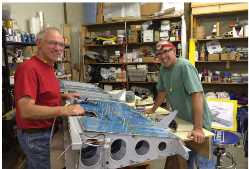
Riveting the wing skins
