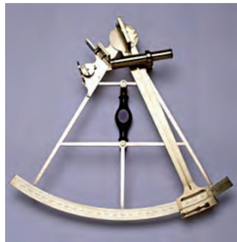
This sextant was made in the late 18th century, but they first appeared in the 1760s. They measured latitude by measuring the sun's distance from the horizon, and calculated longitude by measuring the angle between the moon and stars.
