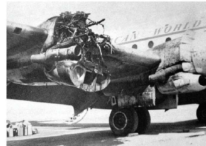
The Pan Am Skipper of this B-377 stated that after an intense struggle, his first officer was finally able to regain roll control of the stricken ship after they came up with the idea to dump fuel from the right wing tanks.
