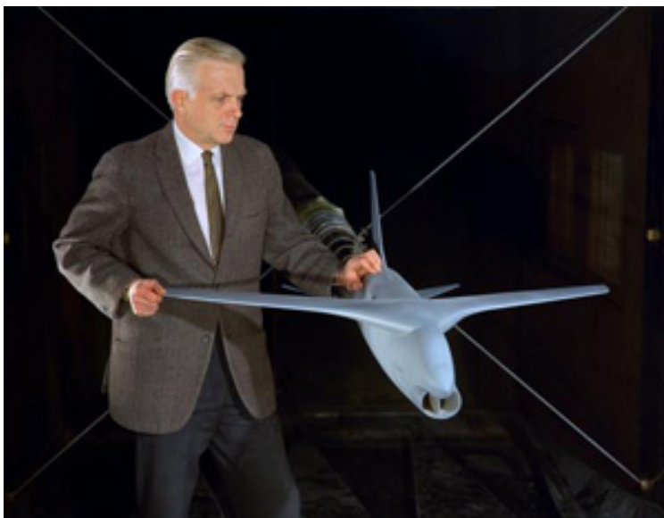
Whitcomb with a wind tunnel model of a TF-8 configured with his supercritical wing, and NASA’s flying version. His innovation has saved billions of dollars in fuel costs. (NASA photo)
