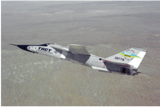
A swing-wing Transonic Aircraft Technology (TACT) F-111A configured with Whitcomb's supercritical wing. It delivered 50 percent better lift than the standard F-111A. (NASA photo)
