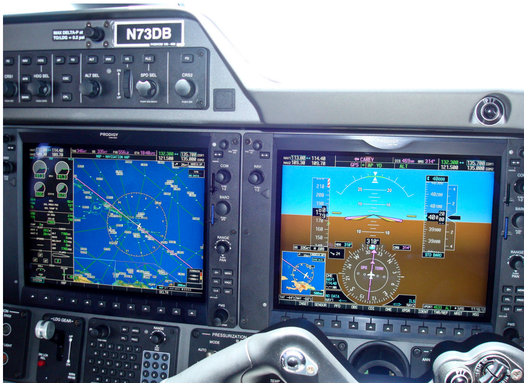
The MFD and my PFD. We are cruising at 40,000 feet north of Hispaniola.
